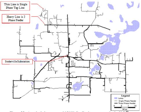
Figure 23. A typical above ground 15 kV distribution geometry in the U.S.<sup>85</sup>
