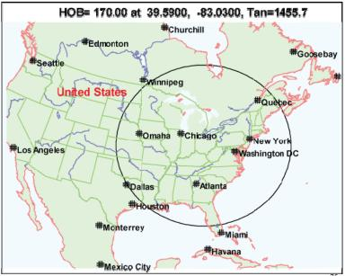
Figure 16: Exposure area for E1 HEMP burst at 170 km over Ohio.<sup>75</sup>
