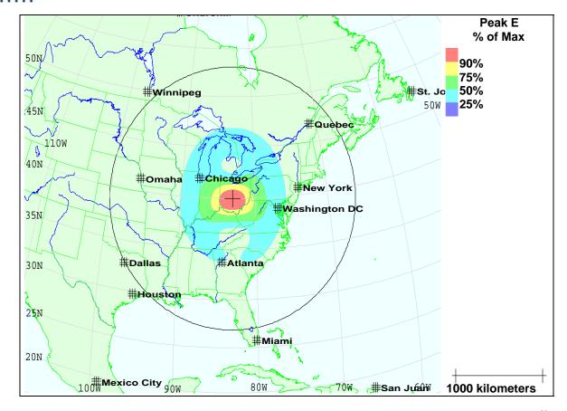
Figure 19: A map showing the E3 Field Pattern from a Large Yield Device positioned over Columbus OH.<sup>80</sup>
