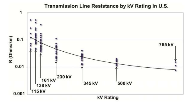
Figure 8: Range of transmission line resistance for the major kV-Rating classes for transmission lines in the U.S. electric power grid infrastructure population. Also shown is a trend line of resistance weighted to population averages. The lower R for the higher voltage lines will also cause proportionately larger GIC flows in this portion of the power grid. (Derived from data in EHV Transmission Line Reference Book and from U.S. DOE-Energy Information Agency and FERC Form 1 Database)
