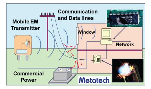
Figure 22: Coupling paths for radiated IEMI fields<sup>84</sup>
