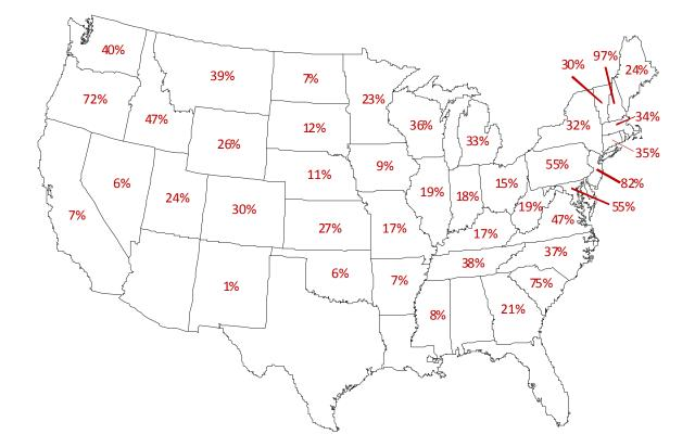
Figure 12: A map showing the At-Risk EHV Transformer Capacity by State for this disturbance scenario, regions with high percentages could experience long duration outages that could extend multiple years.<sup>63</sup>
