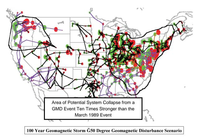
Figure 11: The simulation results showing the pattern of GIC flows in the U.S, grid for a 4800 nT/min geomagnetic field disturbance at  $50^{\circ}$  geomagnetic latitude. The above regions outlined are susceptible to system collapse due to the effects of the GIC<sup>62</sup>
