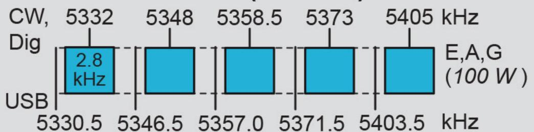
General, Advanced, and Amateur Extra licensees may operate on these five channels on a secondary basis with a maximum effective radiated power (ERP) of 100 W PEP relative to a half-wave dipole. Permitted operating modes include upper sideband voice (USB), CW, RTTY, PSK31 and other digital modes such as PACTOR III. Only one signal at a time is permitted on any channel.
